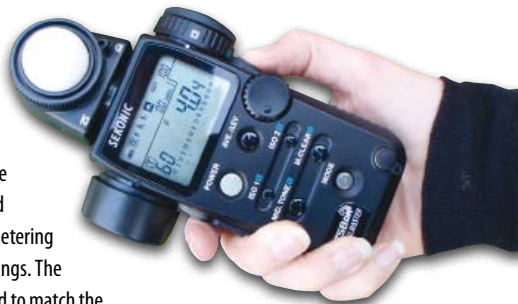
The optical viewfinder on the Sekonic L-758DR displays the reflected light reading through the eyepiece
